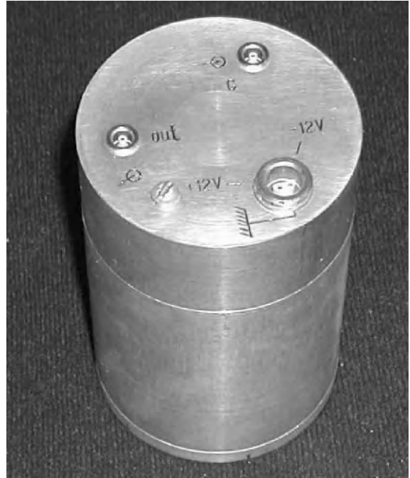
Fig. 1. The prototype 100 \text{ cm}^3 CsI spherical detector.
