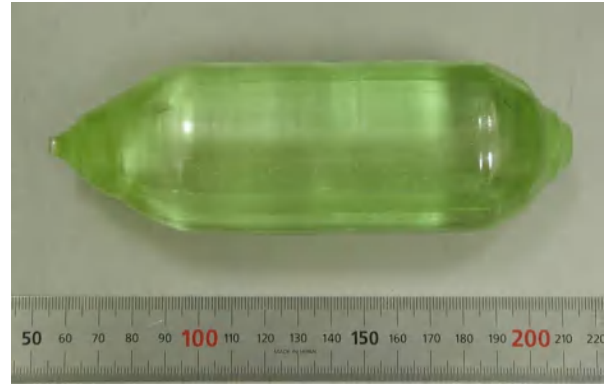
Fig. 1. Pr2.5%:LuAG single crystal with a diameter of 2 inches grown by the CZ method.
