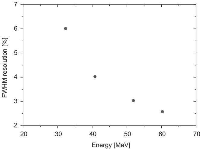
Fig. 7. Measured FWHM resolution vs. proton energy.
