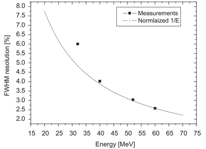
Fig. 9. Measured FWHM resolution and 1/energy curve.
