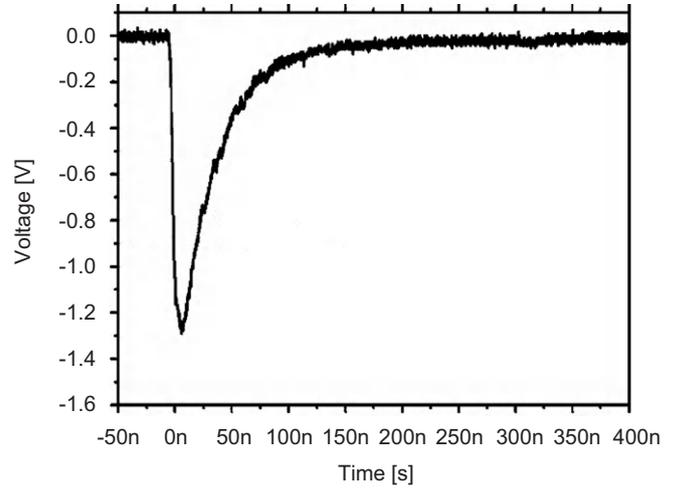
Fig. 5. PMT output signal at 60 MeV.
