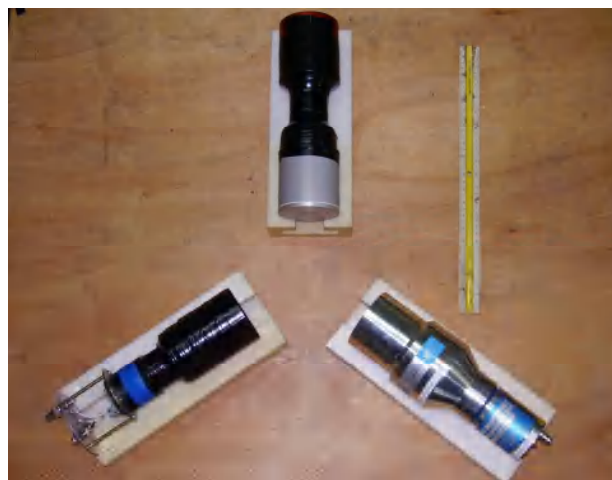
Fig.1. The photograph of the three tested detectors: NaI(Tl) (top), LaBr 3 (right), BGO (left).
