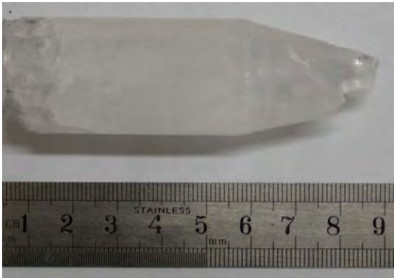
Fig. 1. As-grown \text{LaCl}_3 crystal by Modified Bridgman Method.
